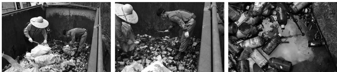
Fig. 1. Crushing process of pesticide bottles in the arm-roll box.
