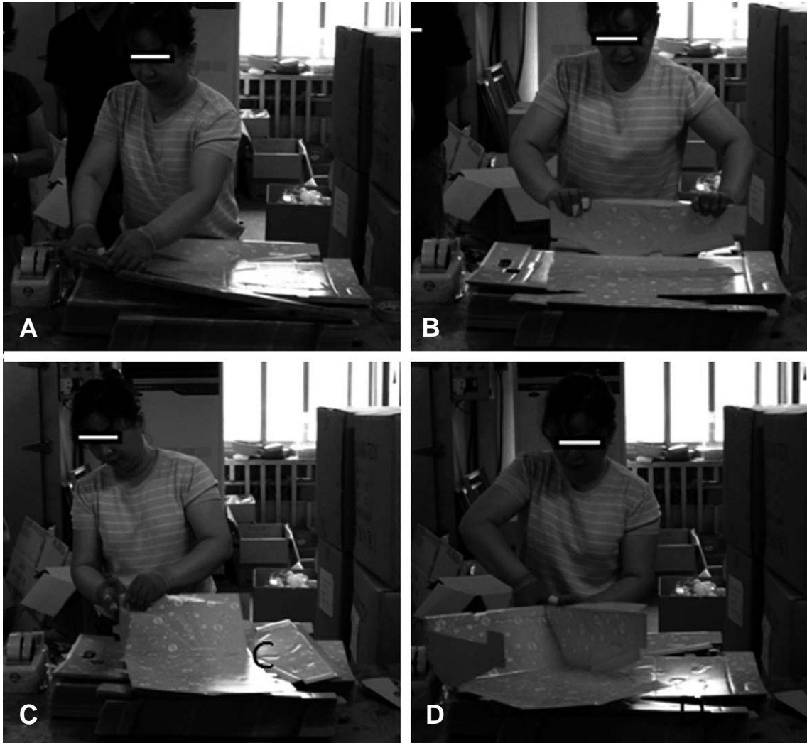
Fig. 3. Folding a A-type box (A) punching, (B) creating three-dimensional shapes, (C) hitting with palm, (D) taping up).
