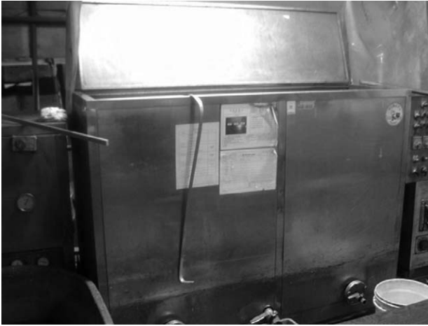
Fig. 1. Degreasing bath with cover using trichloroethylene (TCE).
