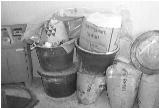
**Fig. 1.** The lead stearate is stored at the corner. It was not closed.
