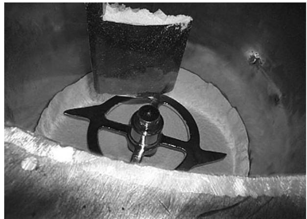
**Fig. 2.** The mixture machine and injected lead stearate.
