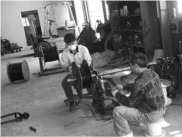
Fig. 5. Rolling the wire ropes on machine for reeling.
