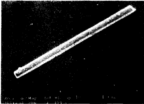
Fig. 3. A scanning electron microscopy shows a glass fiber. It has a smooth and parallel diameter with fractured ends ( \times 400 ).
