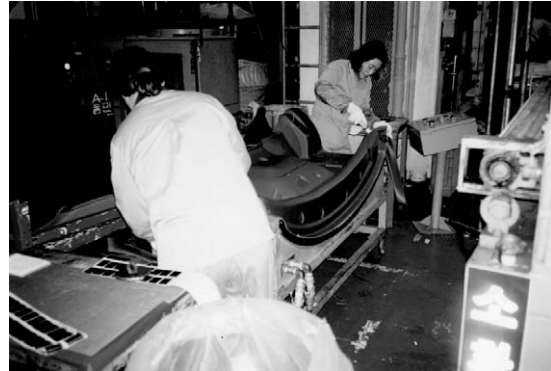
Fig. 2. Vacuum molding process(2)
