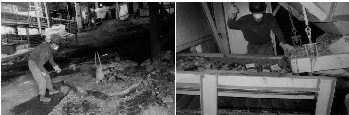
Fig. 1. Giving the calcium carbide stones a good bash with his 3 kg weighted sledgehammer(left) and beating down a lump of manganese with his hammer for making them into smaller sizes(right).
