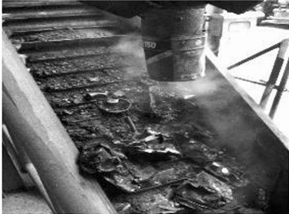
**Fig. 4.** Burnt debris being transported over an apron conveyor.
